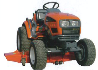
Mid-mounted Jet available for Kioti 'CK' Series tractors – side or rear discharge
