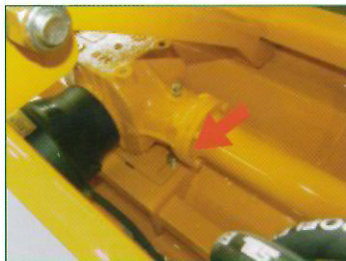
Adjustable skid under the gearbox.
