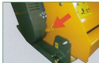
Gearbox with outward greaser.
