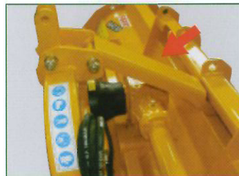
Anti roll bar of the 3.point hitch with bearings (it permits the 3.point displacement and shock-resistant during road transport).
