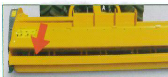
Rear tubular as machine reinforcement. It is used also as anchoring of wheels (option).
