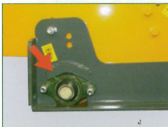
Rear roller adjustable in 6 different positions.
