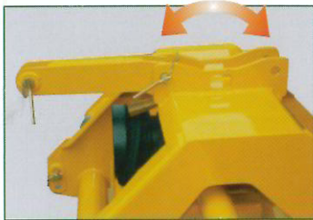
Revolving upper 3 point linkage for front and rear mounting.
