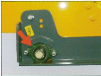
Rear roller adjustable in 6 different positions.
