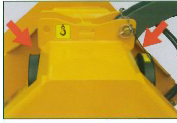
Gearbox prearranged for rear (clockwise rotation) and front (underclockwise rotation) mounting.
