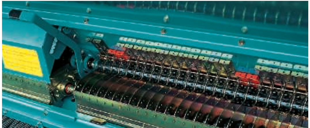
Each row of the SULKY metering system consists of a peg wheel attached to a shaft mounted on ball bearings, an independent shutter, a flap that can be adjusted to match seed size and the REGULINE rotary mechanism.
