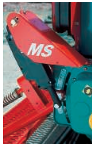
ULTRON MS and SPB VISION : For the rate variator, an electric actuator (with position sensor) is operated from within the cab via the control box.
