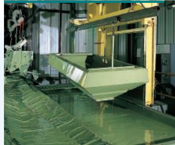
An important stage in the new SULKY anti-corrosion process : components are dipped by robot into a bath of primer.
