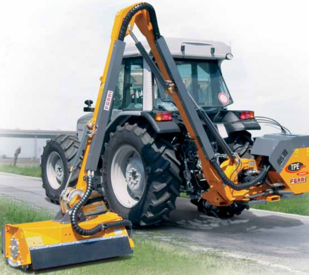
Drop forged arm pivots and flail head linkage.
